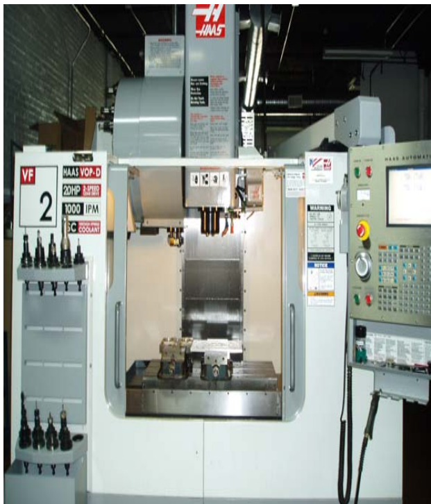
(Vertical Maching Centre ( HAAS Make 20 Tools , 40 Tools Capacity )
